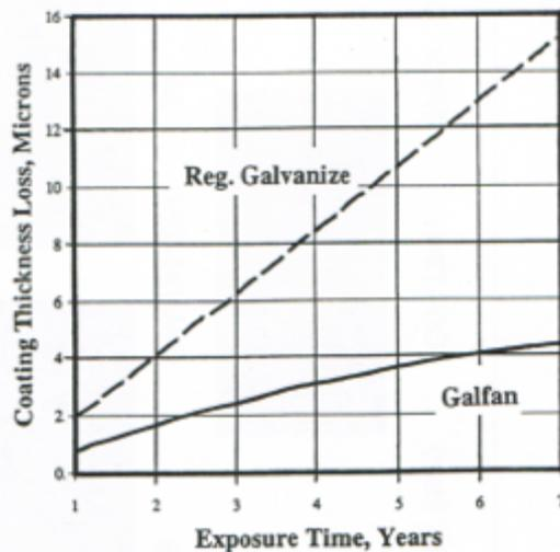
**Figure 2 Coating Thickness Loss in Marine Environment from New Zealand Steel Study<sup>1</sup>**
