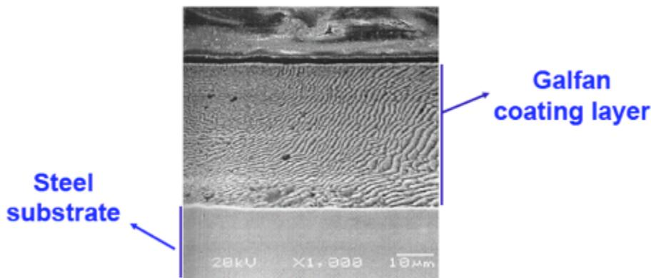
**Figure 1 Microstructure of Zn-5% Al Coating (note the lamellar plate-like structure)<sup>1</sup>**
